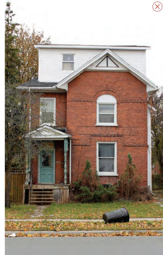
Do NOT: addition alters basic shape of building, and material is not complimentary. Window does not fit with the size and location of other windows.
